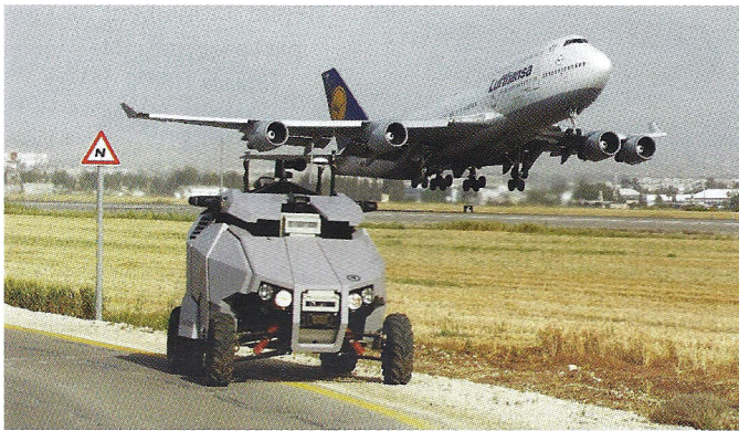
Guardium is claimed to be the first operationally deployed autonomous UGV system
